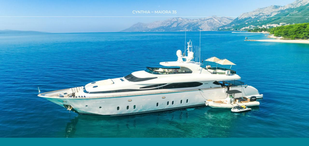
Loa **35.20 m (115' 6")** Beam **7.00 m (23')** Draft **2.7 m (8' 10")** Built **2010** Refit **2024** Guests **8** Crew **6**Builder **Maiora** Naval Architect **Next Yacht Group** Hull Material **GRP** Hull Configuration **Planing hull** Superstructure **Flybridge**
