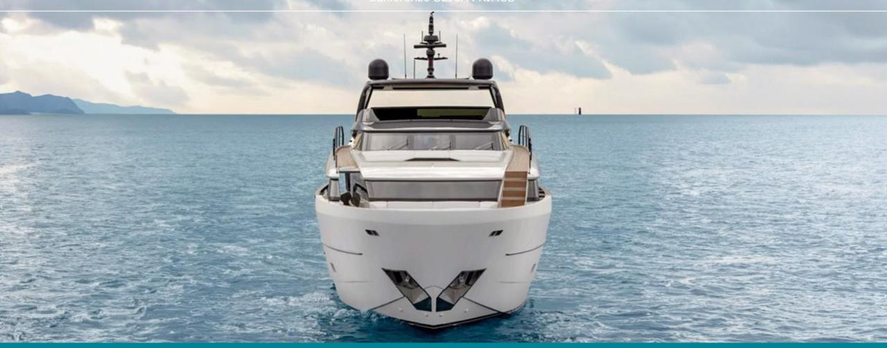
Loa **29.06 m (95' 4")** Beam **6.76 m (22' 2")** Draft **1.9m (6' 3")** Built **2025** Guests **11** Crew **4** Builder Sanlorenzo Hull Material **GRP** Hull Configuration **Planing hull** Superstructure **Raised pilot-house**
