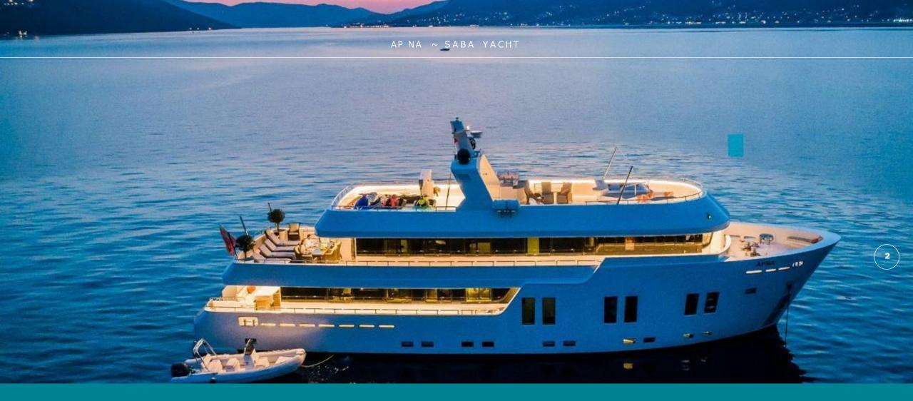
Loa **34.1 m (111'11")** Beam **8.1 m (26' 7")** Draft **2.1 m (6' 11")** Built **2010** Naval Architect **Saba Yacht** Guests **12** Cabins **6** Crew **7** Speed **10 knots**
